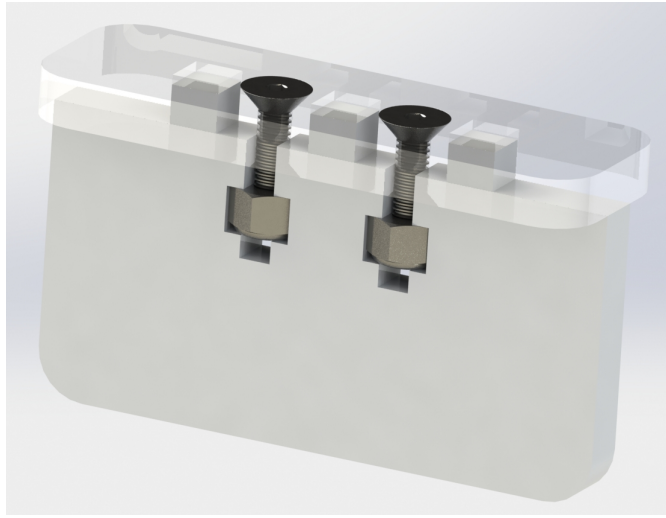
Figure 27: Fastener method used throughout linear book scanner.
